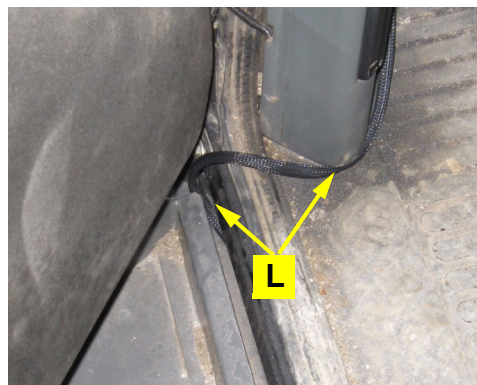
Figure 7: Installed valve control cable
