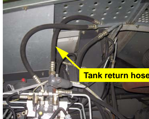
Figure 5b: Installed tank hose for 491 series models
