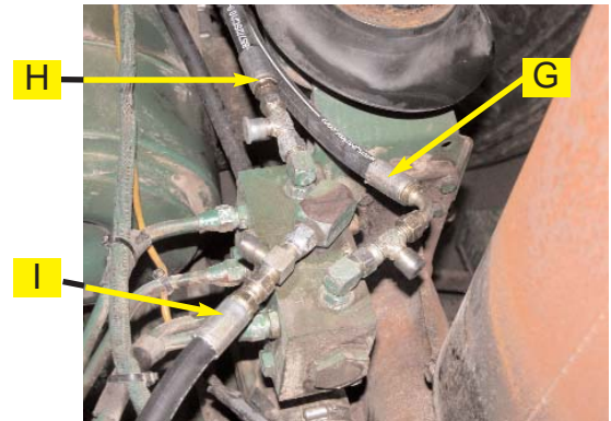
Figure 3g. Tractor Steering Valve with replacement pressure hose ( I ) routed to the front of the tractor.
