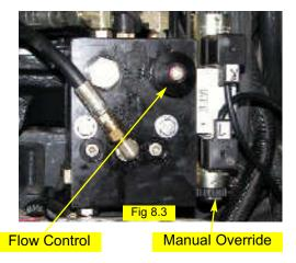
Note: To activate the manual overrides, a tool such as a small screw driver or allen wrench must be inserted into the end of the oil to depress the override button.
