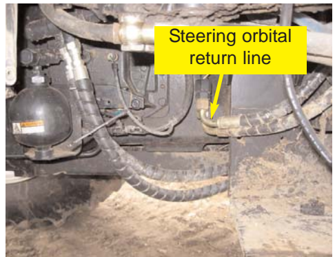
Figure 3b. Pressure and excess flow location.
