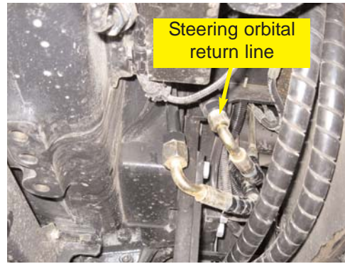
Figure 3a. Pressure and excess flow location.
