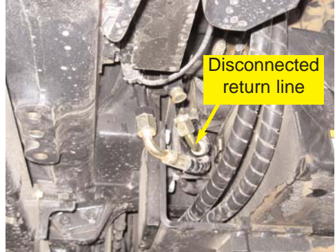
Figure 3c. Disconnected steering return line.
