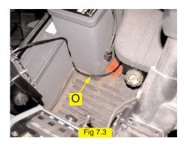
Remove enough slack out of the cable to prevent entanglement with moving parts. Use tie straps as needed.
