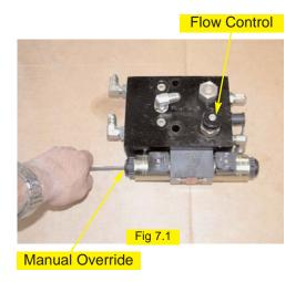
**Note:** To activate the manual overrides, a tool such as a small screw driver or allen wrench must be inserted into the end of the coil to depress the override button.
