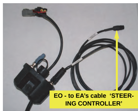
Figure 8e-ii: CAN cable to eDriveX
