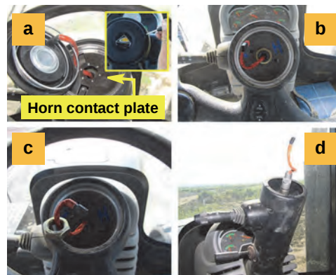
Figures 3-a to 3-d: Removing the horn switch and steering wheel
