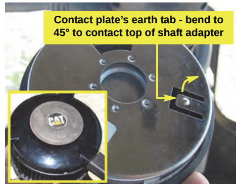
Figure 6b with inset: Adjusting the horn earth tab and installing the center cover
