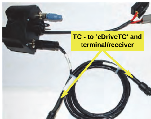
Figure 8e-i: CAN cables to eDriveTC and terminal/receiver
