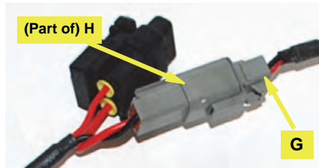
Figure 5c: Power cable to junction box cable
