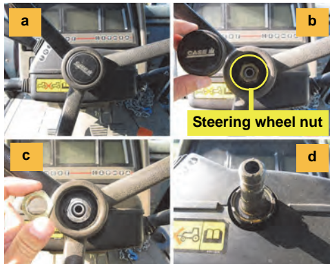
Figure 3 (a-d): Removing the steering wheel
