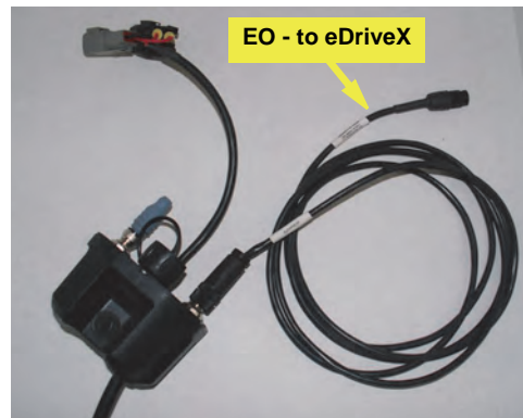
Figure 5e-ii: CAN cable to eDriveX
