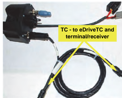
Figure 5e-i: CAN cables to eDriveTC and terminal/receiver
