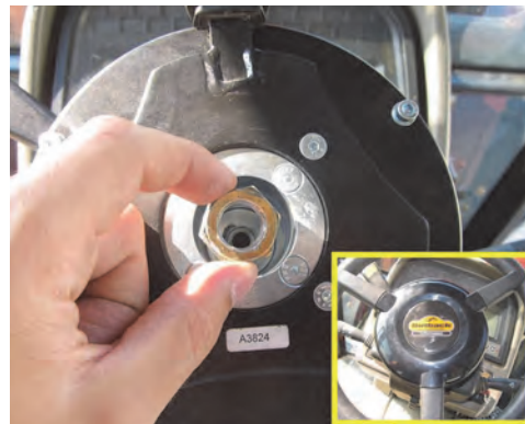
Figure 4b with inset: Steering wheel secured, center cover installed
