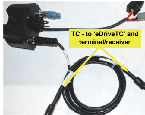
Figure 7e-i: CAN cables to eDriveTC and terminal/receiver
