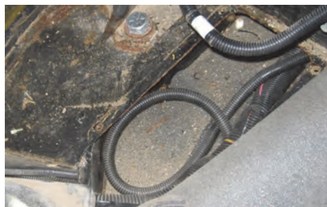
Figure 1: Example pre-drilling check
