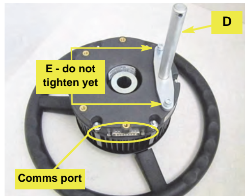
Figure 1c: Anti-rotation T-bar installed
