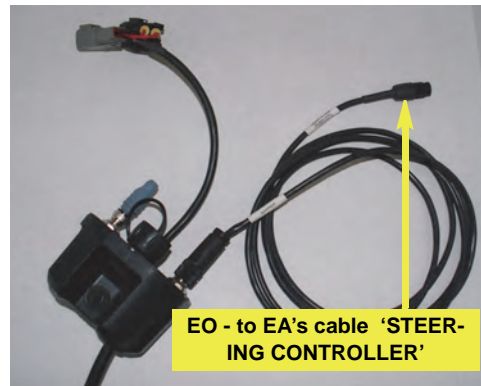
Figure 7e-ii: CAN cable to eDriveX
