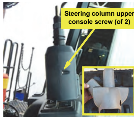
Figure 4a with inset: Removing/reassembling steering column upper console
