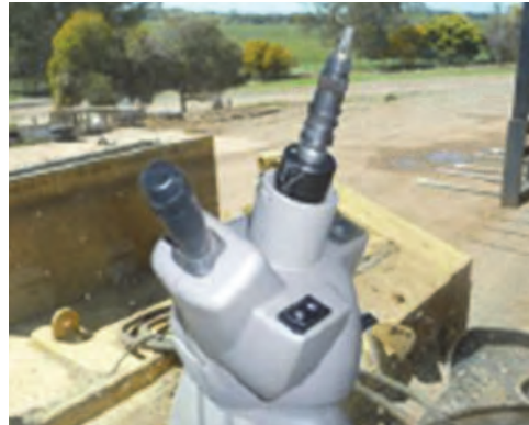
Figure 4c: Reinstalled modified column console
