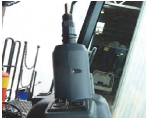
Figure 3b: Steering wheel removed
