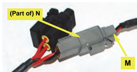
Figure 6c: Power cable to junction box cable
