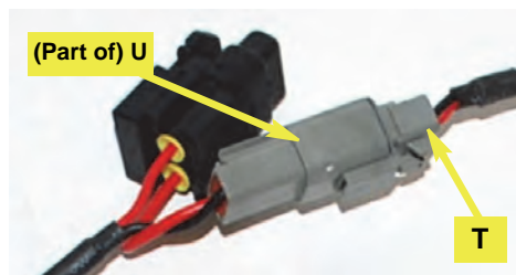
Figure 8c: Power cable to junction box cable
