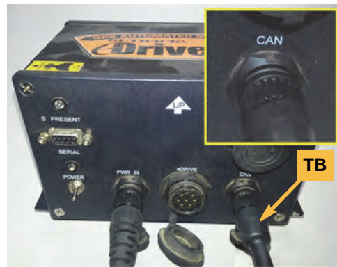
Figure 1c with inset: CAN cable connection at ECU
