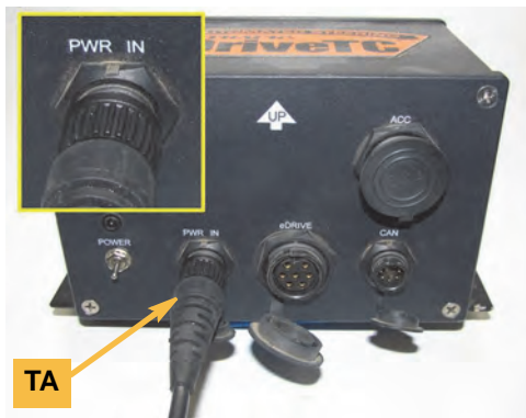
Figure 1b with inset: Power cable connection at ECU
