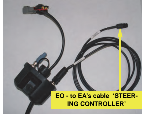
Figure 8e-ii: CAN cable to eDriveX
