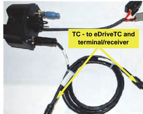
Figure 6e-i: CAN cables to eDriveTC and terminal/receiver
