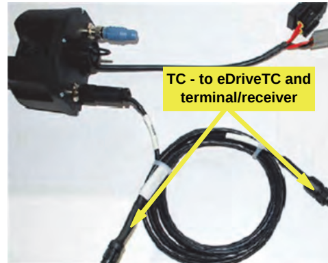
Figure 6e-i: CAN cables to eDriveTC and terminal/receiver
