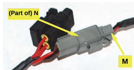
Figure 6c: Power cable to junction box cable
