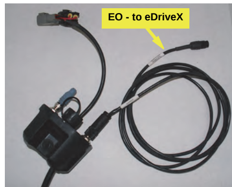
Figure 6e-ii: CAN cable to eDriveX
