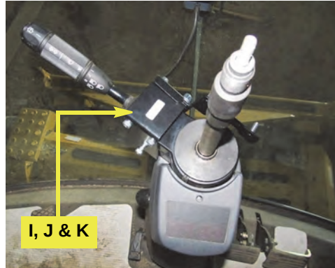
Figure 4a: Anti-rotation assembly installed
