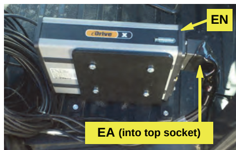
Figure 2a: ECU main cable installed
