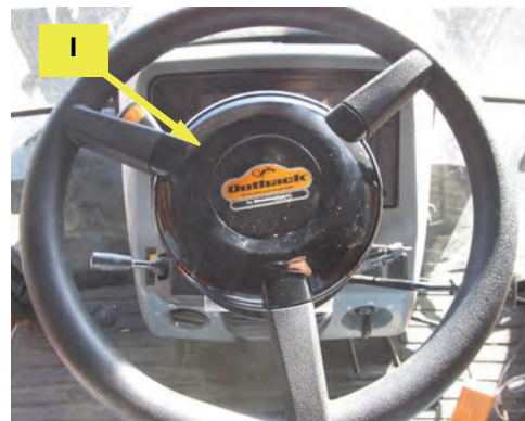
Figure 4c: Center cover installed
