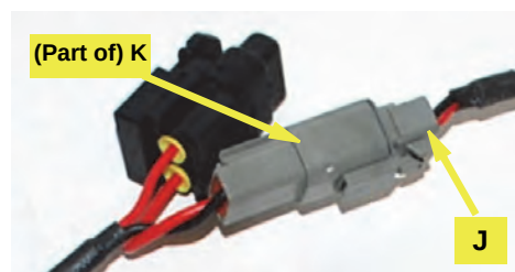
Figure 5c: Power cable connected to junction box cable
