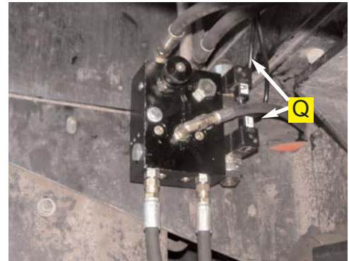
Figure 7a. Valve control cable attached to the Automated Steering Block.
