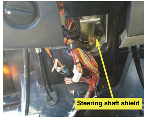
Figure 1: Steering column lower/side console removed, steering shaft shield exposed
