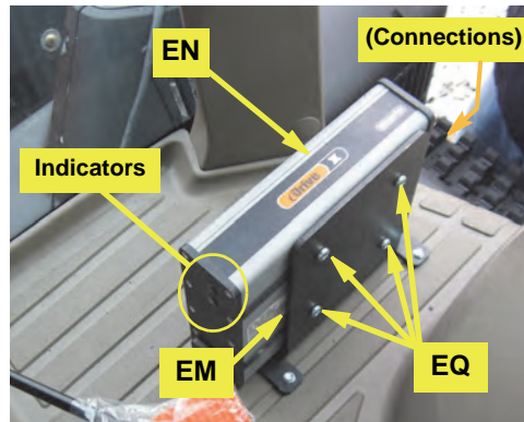
Figure 1b: ECU installed
