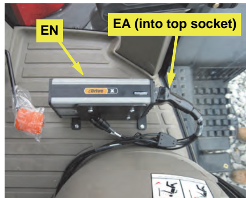
Figure 2a: Installed ECU main cable
