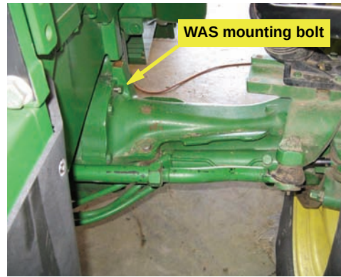
Figure 2a-i: WAS mounting bracket location
