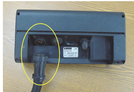
Figure 2: Existing rate controller console cable disconnected
