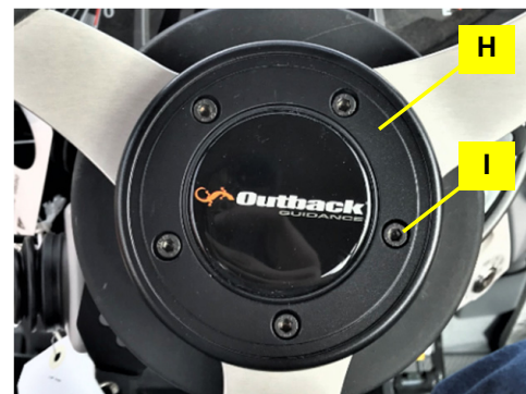
Figure 5: Center cap in wheel
