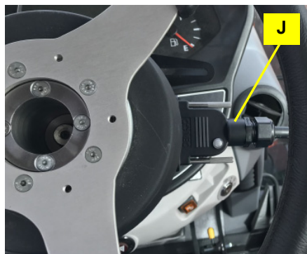
Figure 6: ESi main cable in comms port
