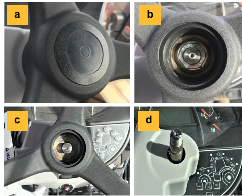
Figures 3a-3d: Removing the horn switch and steering wheel
