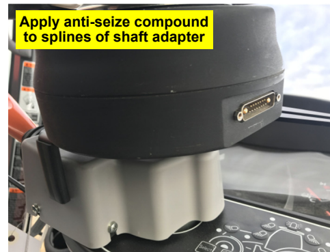
Figure 4a: Wheel assembly installed - comms port to the right
