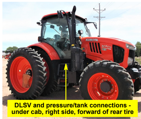
Figure 4b: DLSV and pressure/tank connections access
