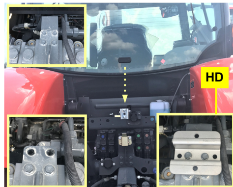
Figure 2 with insets: Steering block mounting bracket location and installation
