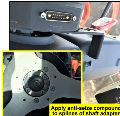
Figure 4a: Wheel assembly installed - comms port to the front
