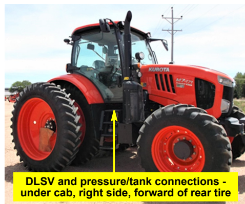
Figure 4b: DLSV and pressure/tank connections access
