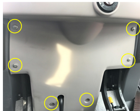
Figure 2b: Console's front cover's six screws
