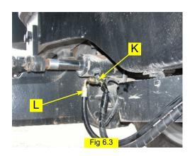
Route the steering hoses back with the tractor steering lines then under the tractor cab and back to the hydraulic control block. For easier routing, the hoses should be routed on opposite sides of the tractor frame before meeting at the hydraulic control block. (Figure 6.4, 6.5, and 6.6) The hoses should be secured with heavy tie straps (provided) to other tractor plumbing. Connect the steering hoses to the **A** and **B** ports of the hydraulic control block as shown. (Figure 6.2)
