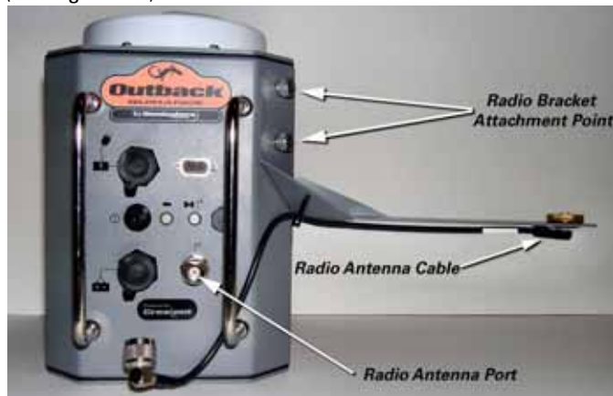
Figure 2-4. Antenna cable bracket attached
