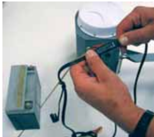
Figure 2-15. External battery cable to the standard power cable
