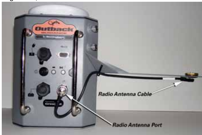
Figure 2-5. Antenna cable attached
