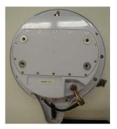
3. Place the faceplate (lip pointing away from unit) on the washers so the holes line up and then secure the faceplate with the provided screws.
