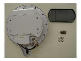
2. Place the four washers over the four mounting holes.
