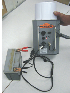
Figure 2-17. Base station connected to the battery
