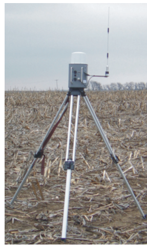
Figure 2-1. Base station on tripod
