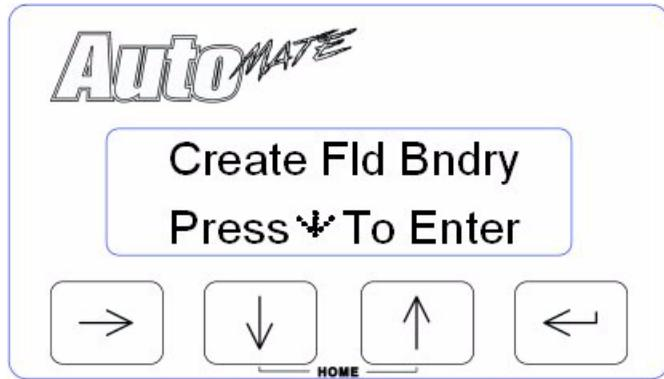
The Create Field Boundary menu enables you to create or replace a no-spray/no plant field boundary while making the first pass around the field. The following screens are available from the Field Boundary menu:
