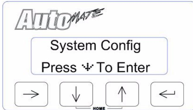
The System Configuration menu allow you to adjust controller settings, such as lighting and unit measurement display. The following screens are available from the System Configuration menu:
