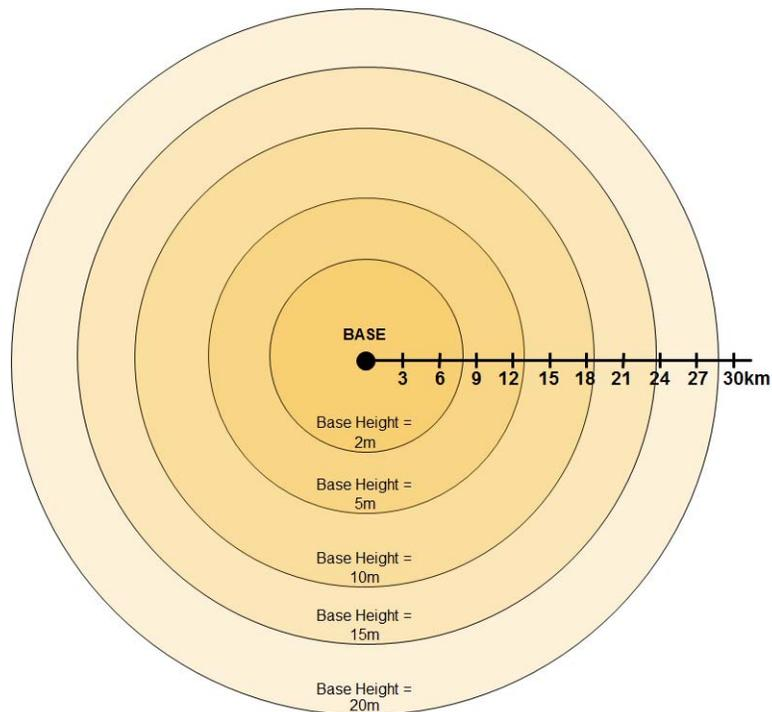
**Figure 3: Typical RTK distance performance vs. base station antenna height above ground**
