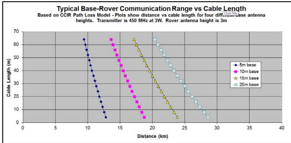
**Figure 4: Typical RTK distance performance vs. RF cable length at base station for four base station antenna heights above ground**
