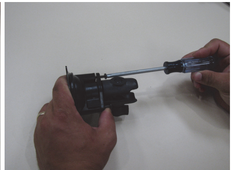
Step 3: Assemble suction cup mount
