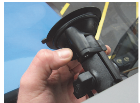
Steps 5/6: Attach suction cup mount to mounting location and tighten
