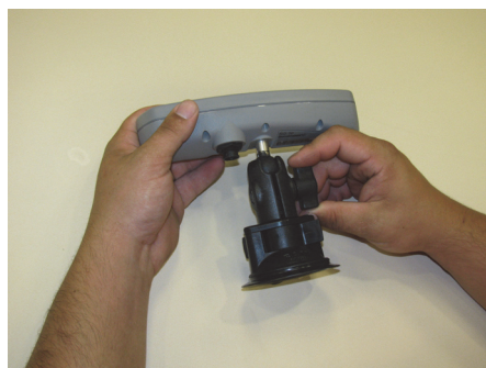
Step 4: Attach suction cup mount to RAM ball and tighten
