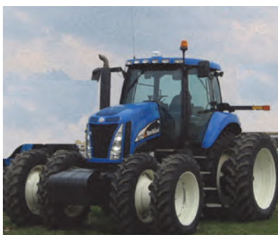
Figure B-4: Machine ballasted with full set of front suitcase weights and rear wheel weights. Wide stance with duals front and rear for stability and traction
