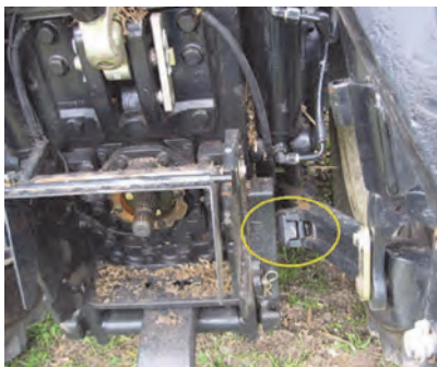
Figure B-5: Vehicle 3-point sway block set tight and spaced evenly on both sides
