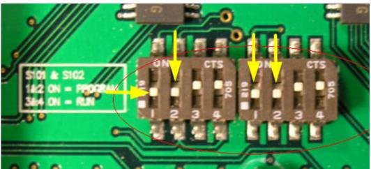
**Step 14** With the side and back panel still off, power up the Outback S-Lite and connect the Outback S-Lite to your computer with a serial cable.
