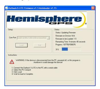
**Step 8** The Outback S-Lite will automatically reboot after loading. Ensure the load has taken effect by checking the software version on the console.
