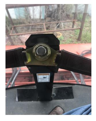
Follow manufacturer's guide to remove steering wheel. SAVE steering wheel nut as it will be reused later in this installation.
