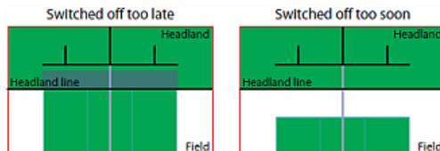
**Off Time** - Enter the number of seconds needed to close the boom valves ahead of a previously applied area. Increase the number to turn off sooner.
