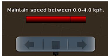
4. Press the left arrow and verify the vehicle steers to the left. Press the stop button (square middle button) as soon as the direction is confirmed.
