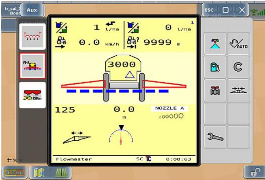
When you connect an ISOBUS-enabled implement to REBEL the implement's information appears in the ISOUT window (see figure above).
