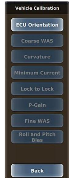
2. Press **ECU Orientation** to display the ECU Orientation panel (see below). When the panel first appears, the Apply Changes button and the Results section are not visible—they appear only after you select values for Logo and Connectors.
