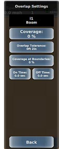
**On Time** - Enter the number of seconds needed to open the boom valves and build pressure ahead of an unapplied area. Increase the number to turn on sooner.
