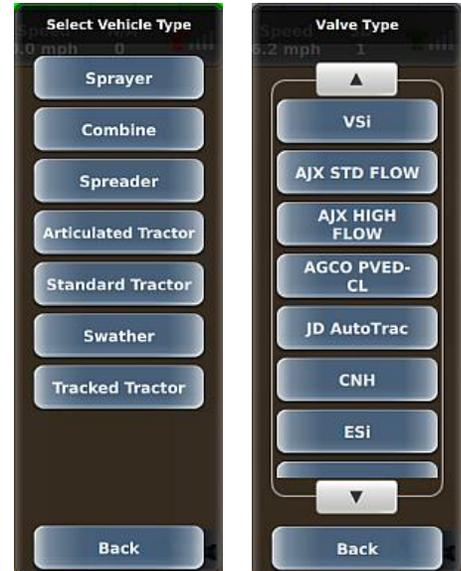
*Note: You can change vehicle type and/or valve type, and upon changing either, REBEL prompts you to restart the ECU for the changes to take effect. Press **OK** to acknowledge the message and continue. Only valve types valid for the currently selected vehicle type are available for selection. If you change the vehicle type and the currently selected valve type is not valid for that vehicle, a valve type no longer appears on the Valve Type button and you need to reselect a valve.*
