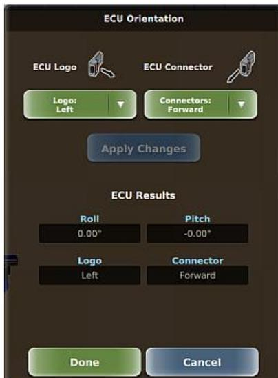
Using the **Logo** and **Connectors** buttons, set the orientation of the top of the ECU (the face with the product logo) and of the two connectors. The connector orientation options are dependent on the Logo orientation so set Logo first. Press **Apply Changes**, then press **Done**.
