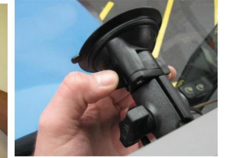
Steps 4/5: Attach suction cup mount to mounting location and tighten
