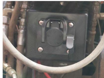
5. Connect the 4-pin Deutsch connector on the retrofit kit to the 4-pin Deutsch connector on the COM2 cable.
