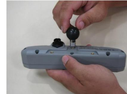
Step 1: Attach mounting ball to lightbar
