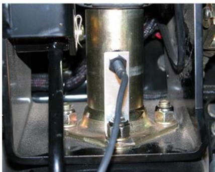
**Example C (CSTX-2, wheel machines):** This installation required only minor modification of the switch bracket (drill and bend). The bracket is mounted on an existing stud.
