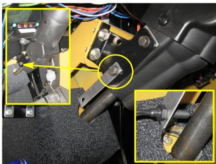
**Example B (SC4640):** This installation mounted the slightly modified bracket (drilled) using an existing bolt in a steering column support bracket.
