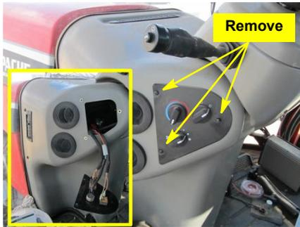
**Example A (AP20AS):** The AP20AS models have only limited access to the steering shaft without major dismantling of the steering column enclosure. You can, however, access the steering shaft through the opening behind the climate control knobs. Inside the enclosure, you can manipulate the magnets and the switch sensor into position on and near the shaft respectively (see picture at right) without a clear view of the shaft and the items you are placing.
