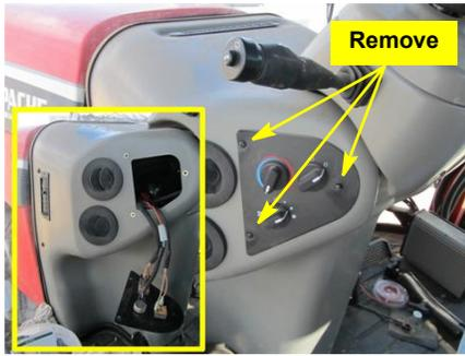
**Example A (AP20AS):** The AP20AS models have only limited access to the steering shaft without major dismantling of the steering column enclosure. You can, however, access the steering shaft through the opening behind the climate control knobs. Inside the enclosure, you can manipulate the magnets and the switch sensor into position on and near the shaft respectively (see picture at right) without a clear view of the shaft and the items you are placing.
