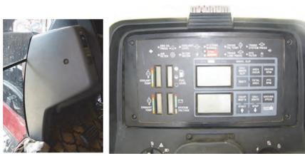
**Example E (CASE C8900-A):** This installation required removal of the steering console side panels (far left) and the electronic instrument cluster (left). Exposed steering shaft at right.
