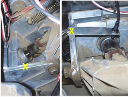
**Example E (CASE C8900-A):** This installation did not require modification of the switch bracket. But it did require use of some of the magnets' epoxy to stick the switch bracket to the (thoroughly cleaned) cast alloy steering column mounting.
