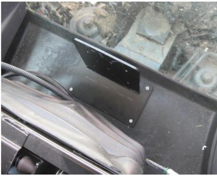
**Example E (MF8600):** This installation used the ‘slanted’ floor bracket (> 90°, labeled B in B2 on page 2). Floor space restrictions dictated that the bracket/ECU be mounted behind the driver’s seat. The bracket’s long sides are perpendicular to the machine’s fore/aft center-line. The slanted mounting face compensates for the mounting platform’s dip toward the back of the seat. The ECU top (ribbed, labeled face) will be forward and the connector to left or right.
