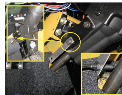
**Example B (SC4640):** This installation mounted the slightly modified bracket (drilled) using an existing bolt in a steering column support bracket.
