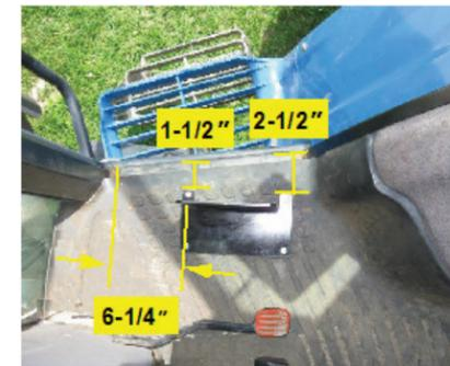
**Example B (NH8070):** Underfloor clearance requirements dictated that the bracket be installed in this cab area. The bracket is set with its long side parallel to the machine's fore/aft centerline.
