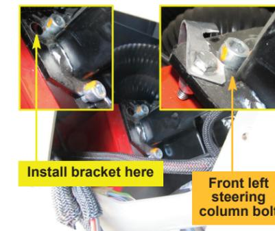
**Example A (AP20AS):** In this installation you install the modified switch bracket (at right—drilled, cut, twisted and bent) in the spare hole beside the left front steering column bolt (at left) inside the steering column enclosure accessed through the opening behind the climate controls panel (see Example A in Table C2-1).
