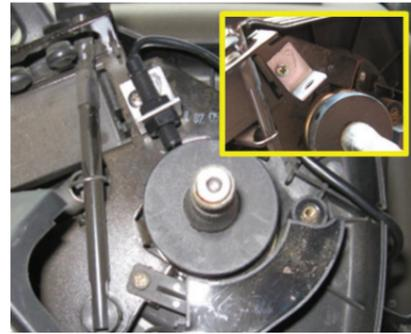
**Example D (CSTX-2, Quadtrac machines):** This installation required cutting, drilling and bending. The bracket is mounted using an existing screw.
