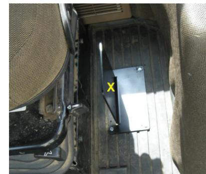
**Example A (JD8000):** The 90° floor-mounted bracket (labeled A in B2 on page 2) is the most commonly used ECU bracket. In this installation, the bracket is mounted to the left of the driver's seat on the cab floor. The one-inch tabs are toward the driver's seat and the bracket is set with its long side parallel to the machine's fore/aft centerline.
