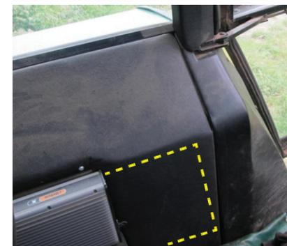
**Example D (JD4040 and JD7010, standard [non-articulated] machines—eDriveX installation shown):** With no suitable floor space available, the 'flat' bracket (labeled C in B2 on page 2—provided as required) is used. The bracket must be installed with its mounting face ('out-bulge') vertical and its long sides parallel to the floor. (Nuts, bolts and washers will be provided for this 'non-floor' mounted bracket.)
