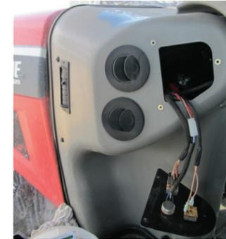
**Example A (AP20AS):** Access the steering shaft through the opening behind the climate control knobs. Inside the enclosure, with the switch bracket temporarily removed, you can manipulate the magnets into position on the shaft.
