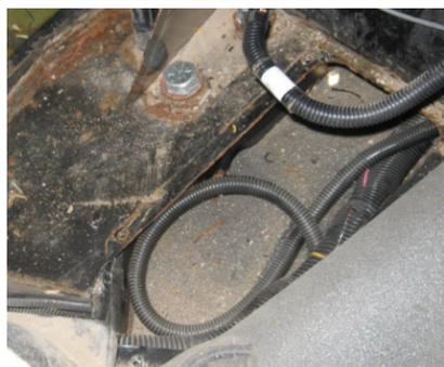
**Example - All installations:** Before drilling (or using self-drilling screws) in the cab, make certain there is nothing that can be damaged by the drilling or by any self-drilling screws used to secure the ECU mounting bracket. Secure anything that could be damaged away from where the screws come through. See figure at left for an example of a pre-drilling check; it shows an under-floor cabling compartment.
