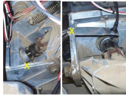
**Example E (CASE C8900-A):** This installation did not require modification of the switch bracket. But it did require use of some of the magnets' epoxy to stick the switch bracket to the (thoroughly cleaned) cast alloy steering column mounting.
