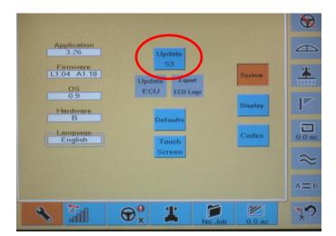
When the USB drive is recognized to have an S3 update available, the Update S3 button will activate (turn blue). Press the Update S3 button in the systems tab, and wait for the load to complete. (After loading, a manual reboot may be necessary if the S3 does not reboot automatically after 5 minutes.) Verify a successful load by checking the Application version has changed to 3.50.14.
