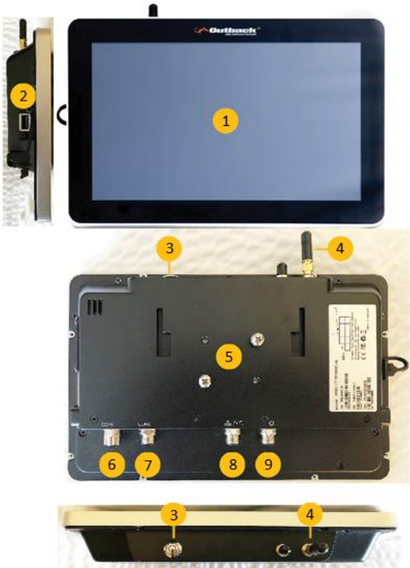
Figure 1-1: MaveriX Terminal front and back views
