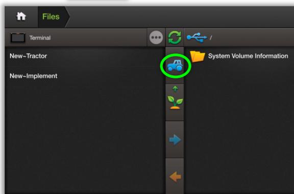
Select a machine from the list on the left and push the blue arrow to backup a profile to USB.
