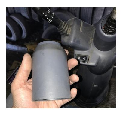
Remove the screws that hold the steering column plastic halves together and **SAVE** to use later in this installation.
