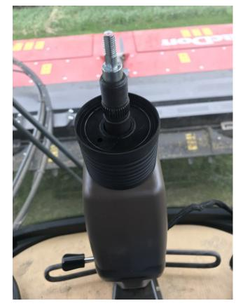
Remove the two screws that hold the plastic cover to the column. Remove and discard the plastic cover.
