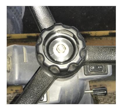
Remove the telescoping actuator knob to gain access to the nut that holds the steering wheel onto the shaft.
