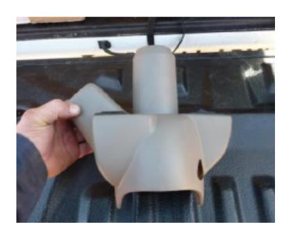
Mark and draw a circle 60mm (2-3/8") up from the base of the plastic column. The line should be just above the screw holes.
