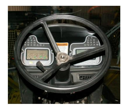
Remove the upper plastic sleeve from the steering column to gain access to the screws to take the steering column plastic apart. Discard plastic sleeve.
