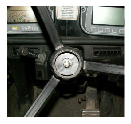
Remove the telescoping actuator knob to gain access to the nut that holds the steering wheel onto the shaft.
