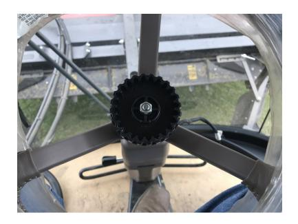
Remove the telescoping actuator knob to gain access to the nut that holds the steering wheel onto the shaft.
