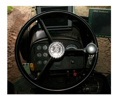
Remove the telescoping actuator knob to gain access to the nut that holds the steering wheel onto the shaft.
