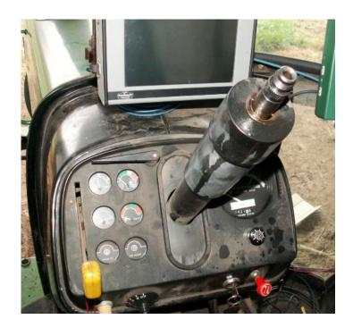
Remove plastic sleeve to gain access to the metal steering column. Discard plastic sleeve. The steering column is now ready for ESi<sup>2</sup> Installation.
