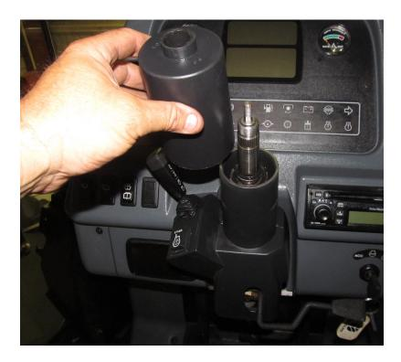
Remove the screws that hold the steering column plastic halves together.
